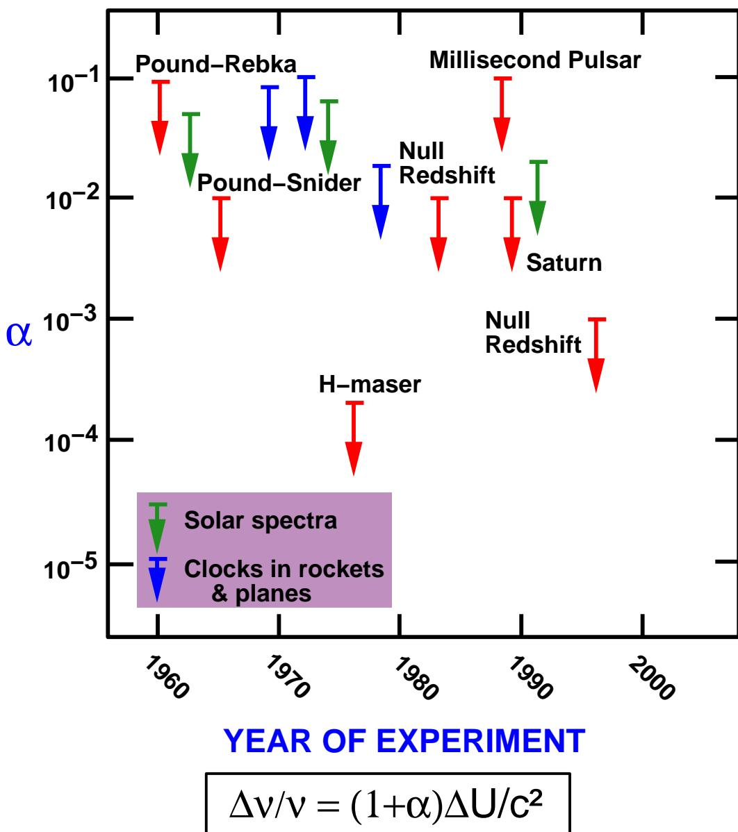
Selected tests of local position invariance via gravitational redshift experiments, showing bounds on  $\alpha$ , which measures degree of deviation of redshift from the formula  $\Delta\nu/\nu = \Delta U/c^2$ .
