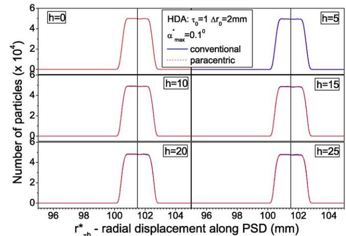
Fig. 8. Line shapes for  $h = 0 - 25$  mm for equal sized ( $\bar{R} = 101.6$  mm) paracentric ( $\xi = 1.2308$  and  $\gamma = 1.5$ ) and conventional ( $\xi = \gamma = 1$ ) HDAs (see Table 1) at  $\tau_0 = 1$  with  $\Delta r_0 = 0.2$  mm (top) and  $\Delta r_0 = 2$  mm (bottom), for  $\alpha_{\max}^* = 0.1^\circ$ . Lines mark the position of the exit of the central ray with  $r_0 = R_0$ ,  $\alpha^* = 0$ .
