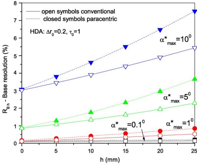
Fig. 6. Comparison of  $h$ -dependence of base resolution  $\mathcal{R}_{Bh}$  for a conventional (open symbols) and paracentric (closed symbols) HDA of equal size ( $\bar{R} = 101.6$  mm) for  $\tau_0 = 1$  and  $\Delta r_0 = 0.2$  mm.
