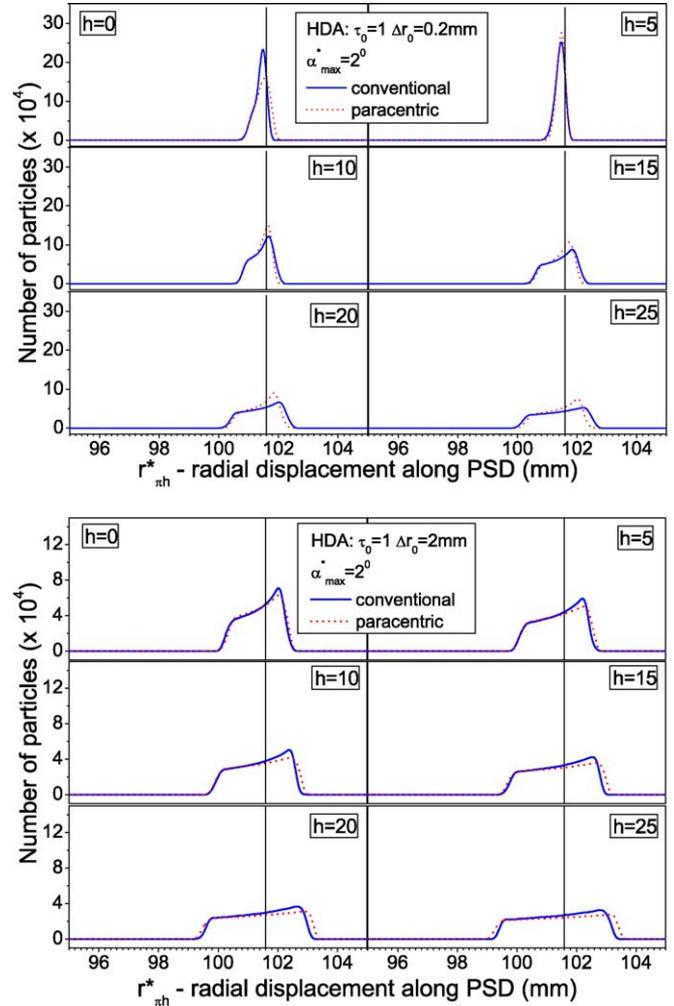
Fig. 10. Same as Fig. 8, but for  $\alpha_{\max}^* = 2^\circ$ . As  $h$  varies from 0–25 mm, for  $\Delta r_0 = 0.2$  mm the biased paracentric HDA has  $\chi_h$  (Eq. (41)) vary from 0.460–5.363, while the conventional HDA has  $\chi_h$  vary from 0.618–4.354. For  $\Delta r_0 = 2$  mm the corresponding  $\chi_h$  variations are 0.08357–0.9753 and 0.1124–0.7919, respectively.
