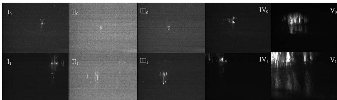
**Fig. 2.** Case study 1: images of groups of carrot sprites as were observed on July 29th, 2005. (I) 01:40:50.204 UT; (II) 01:40:50.246 UT; (III) 01:40:50.287 UT; (IV) 01:40:50.329 UT and (V) 01:40:50.370 UT. For each time two images are presented—the upper (\*.0) for wide FOV and the bottom (\*.1) for narrow FOV.
