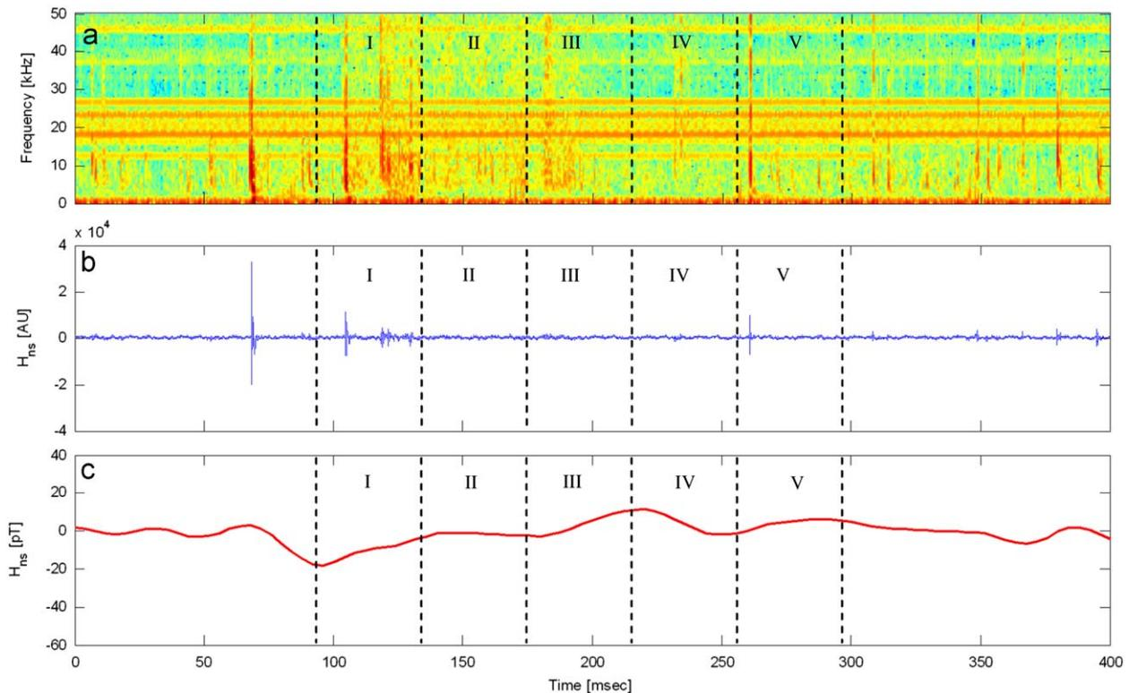
**Fig. 9.** Case study 4: (a) VLF dynamic spectrum, (b) VLF time series and (c) ELF time series associated with the groups of sprites during 400 ms, starting at 01:36:09.300 UT.
