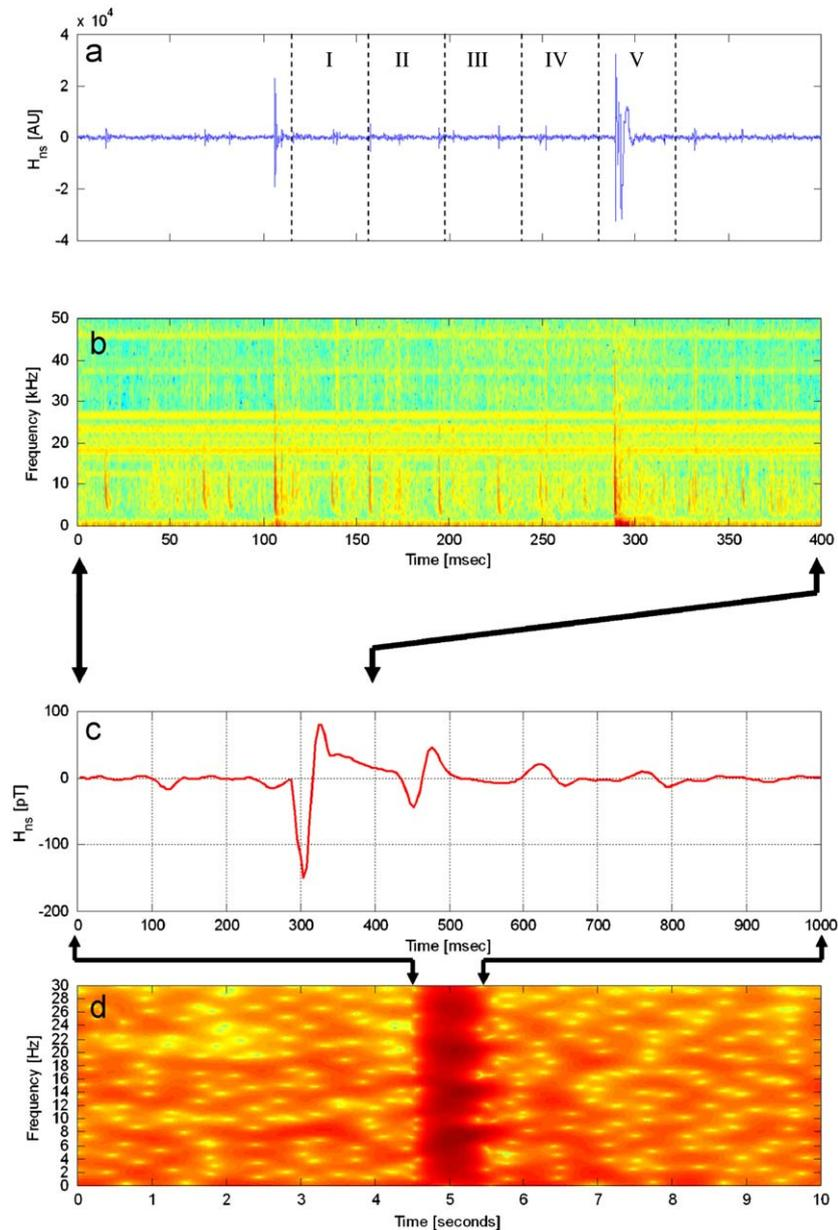
**Fig. 3.** Case study 1: time series and dynamic spectrum of the ELF and VLF signals associated with the groups of sprites as recorded in Israel (MR and SB, respectively),  $\sim 3300$  km from lightning origin. (a) VLF time series starting at 01:40:50.100 UT; (b) VLF dynamic spectrum starting at 01:40:50.100 UT; (c) ELF time series starting at 01:40:50.100 UT and (d) ELF dynamic spectrum starting at 01:40:45.100 UT.
