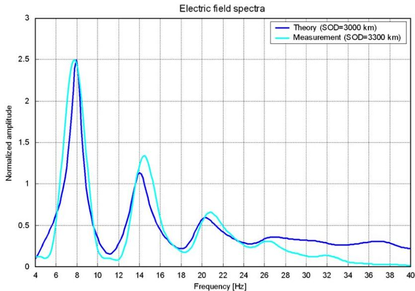
**Fig. 12.** Simulation of the q-TEM mode equations for the electric field component (assuming SOD  $\sim$ 3000 km), and measurement of the signal (actual SOD  $\sim$ 3300 km).
