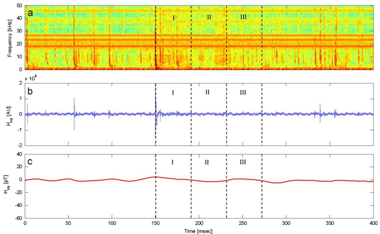
**Fig. 11.** Case study 5: (a) VLF dynamic spectrum, (b) VLF time series and (c) ELF time series associated with the groups of sprites during 400 ms, starting at 01:46:04.600 UT.
